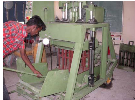
Figure 1. Hollow Blocks with Foundry Waste Sand
